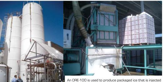
An ORE-100 is used to produce packaged ice that is injected into boxes of broccoli for cooling during transportation.
